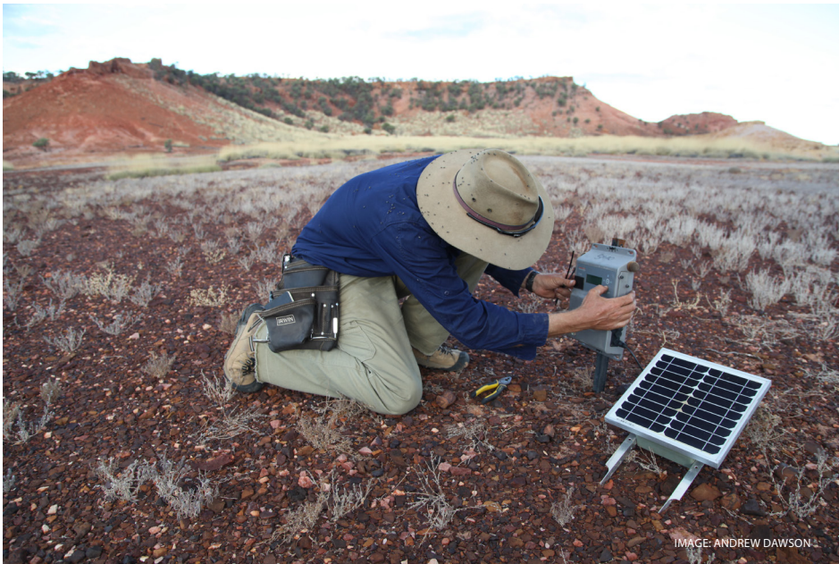
The instrument being set up in the image above is an acoustic recorder. These instruments are an important tool for night-parrot research and are used for both detection and long-term monitoring.
