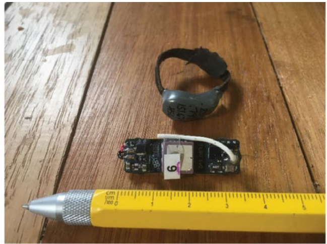
Figure 4: (L) GPS unit circuit board. Electronics cannot be sufficiently flexible to the tight circumference needed to fit around an LBP neck. (R) On the right, comparison of GPS unit and VHF collar showing tight neck circumference.
