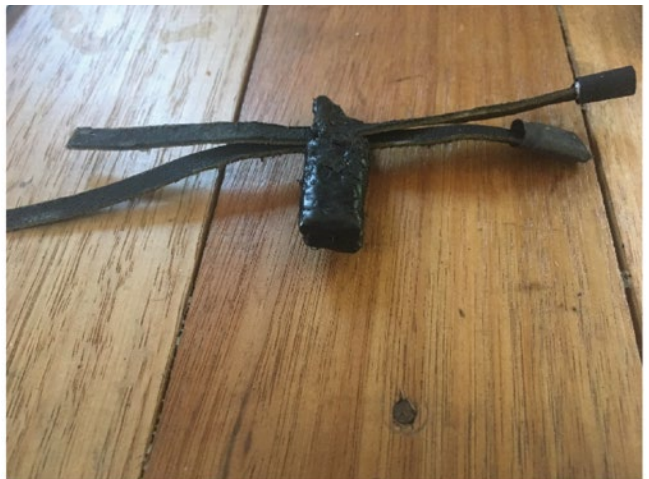
Figure 6: Final harness design, with no neoprene straps. Both straps are made of leather and use a method of attachment that is known to work for conventional radio collars.
