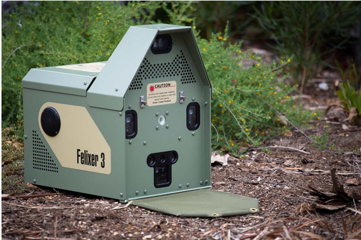
Figure 5: With so few animals surviving extensive fire (and some of those being native predators), control of introduced pest predators is an essential step in the short-term response to fire. Pictured here is the Felixer trap, an innovative device targeting feral cats that depends upon their fastidious grooming behaviour and size and shape detection beams. This is one of a number of innovative approaches that could be rolled out for pest predator control at the interface between burnt areas and unburnt refuges. (Photograph: John Read).
