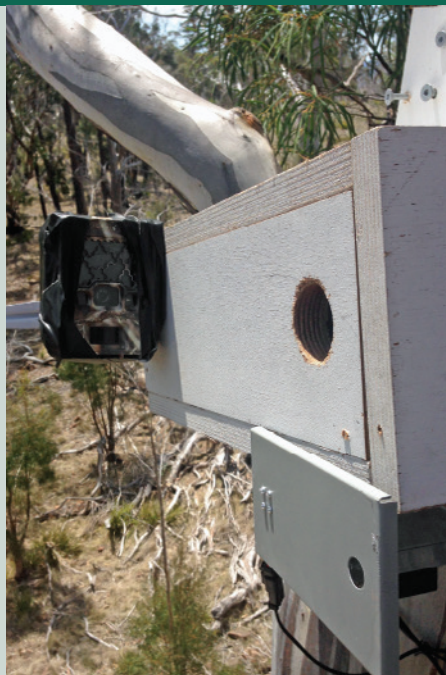
Nest box showing the solar-powered door known as a "possum-keeper-outerer". Photo: Dejan Stojanovic
