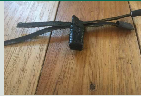
ABOVE: Figure 2: The final harness design, with no neoprene straps. Both straps are made of leather instead, and use a method of attachment that is known to work for conventional radio collars. Image: Lachlan McBurney
