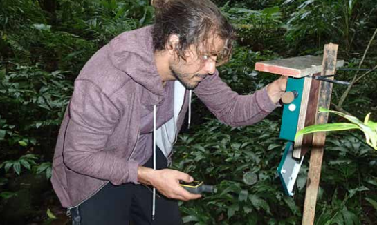
LEFT: Research officer Liam Bolitho deploying a call recorder in the field. Recordings of calling males are used to estimate frog population sizes. Image: David Newell
